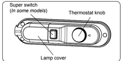
The thermostat automatically regulates the temperature inside the refrigerator and freezer compartments. Cooler temperatures can be obtained by rotating the knob to higher numbers, 1 to 5.
