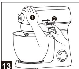
13 Press the head of the mixer, then release the lock lever right.
