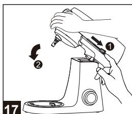
17 Release lock lever right, press down the head of the mixer.
