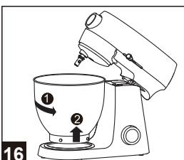
16 Remove attachment by turning the attachment counterclockwise and pull to remove.
